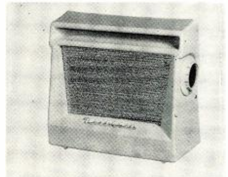
The Heath six-transistor radio receiver, (shown assembled) unlike many other sets of the type, is not subminiaturized.
